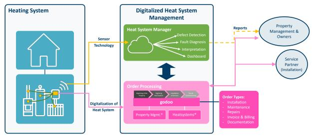
On the basis of this data, evaluation reports including situation analyses, proposed solutions and catalogs of measures are being created. The evaluation of the measurement data allows for determinations such as the **precise power requirement** for the replacement or optimization of the heating system. This results in **reduction of operating costs**, **energy consumption** and **CO**<sub>2</sub> **emissions**, all of which directly benefit the customers.
